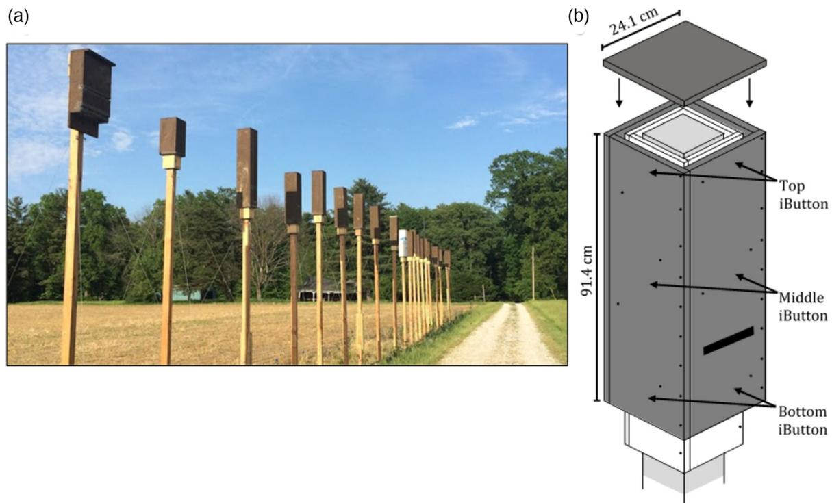
**FIGURE 1** (a) Twenty bat box designs installed in Vigo County, Indiana, May–September 2018. (b) Schematic with dimensions of a reference rocket-style bat box and iButton temperature data logger locations. Data loggers were placed between the outer (dark grey) and inner (white) sleeves. To maintain chamber widths, wooden blocks were placed between the outer and inner sleeves and the post (light grey) and inner sleeve
